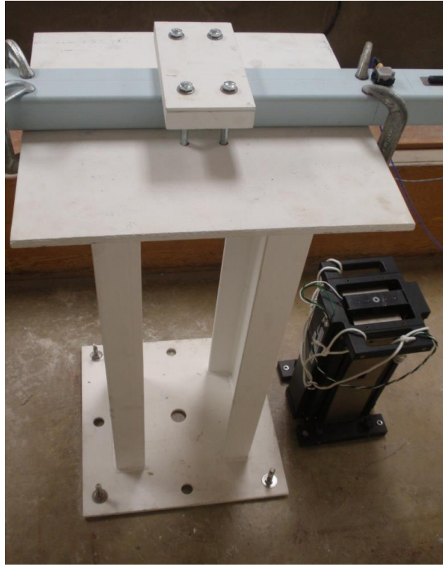
Figure 3.2: Fixed end of HSS cantilever
