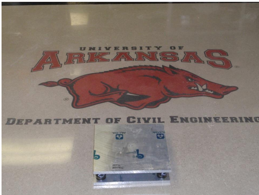
Figure 4.10: Force plate assembly (TecsPak GBA 107s bumpers) with top aluminum plate installed. Photo taken by Jeremy Rawn, Fall 2010 Engineering Research Center
