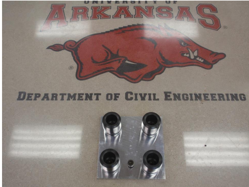
Figure 4.7: Bottom of force plate assembly with TecnPak GBA 119S bumpers at corners (impact force sensor not shown)
