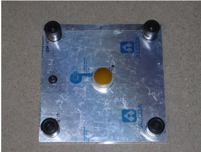
Figure 4.9: Bottom of force plate assembly with TecsPak GBA 107S bumpers (corners) and Model 200C50 impact force sensor (center). Photo taken by Jeremy Rawn, Fall 2010 Engineering Research Center
