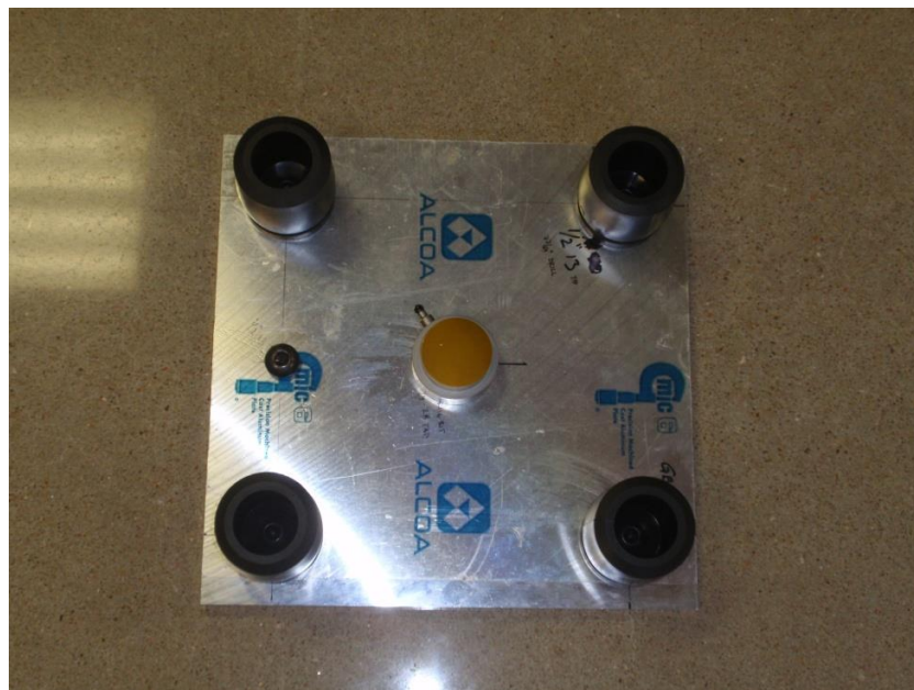
Figure 4.8: Bottom of force plate assembly with TecnPak GBA 113S bumpers (corners) and Model 200C50 impact force sensor (center).
