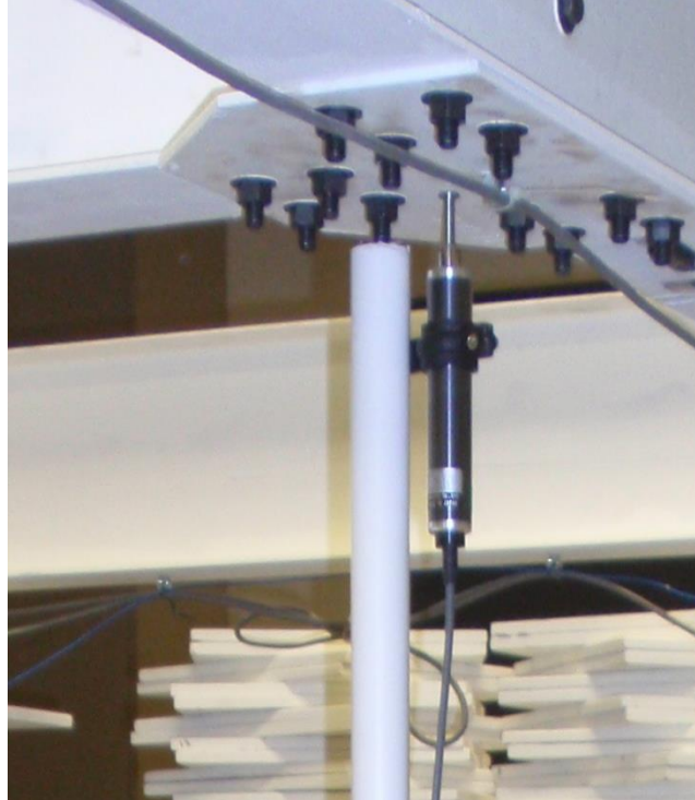
Figure 3.11: TML CDP-25 displacement transducer installed under the grid model structure. Photo Taken by Jason Herrman, Fall 2010 Engineering Research Center
