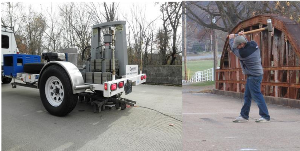
Figure 4.6: Falling Weight Deflectometer with Bumpers below Load Plate and Modal Impact Hammer
